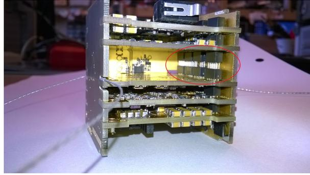
(a) The power bus connecting the internal PCBs.
